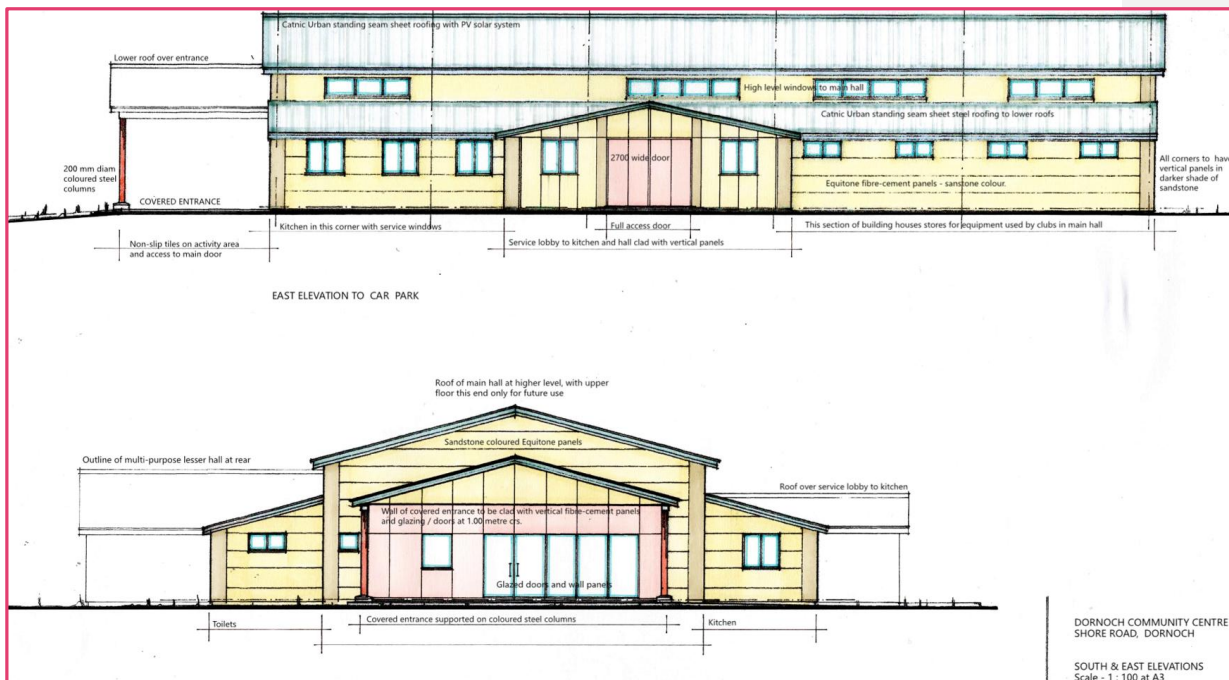
Figure 6: Architect's drawings showing East and South Elevations of the new community centre
